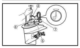
(3) Install the backlash indicator onto the drive shaft (16mm (0.63 in) diameter).
