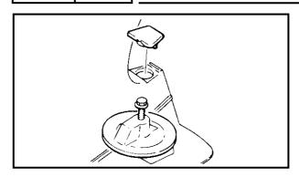
4. Install the trim tab on the gear case. Be sure to align the marks put on both of them when they were removed. Place the cap over the bolt hole.
